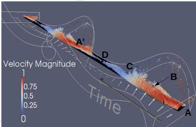
**Fig. 2** Vorticity isocontour colored by scaled velocity magnitude ( $\frac{\sqrt{u^2+v^2}}{\max(\sqrt{u^2+v^2})}$ ). Two periods shown. Arrows indicate incoming angle of attack variation. Points A, A' correspond to  $\alpha = 0$ , B to separation location, and C to reattachment D to minimum angle of attack. White lines show field of view in airfoil fixed frame
