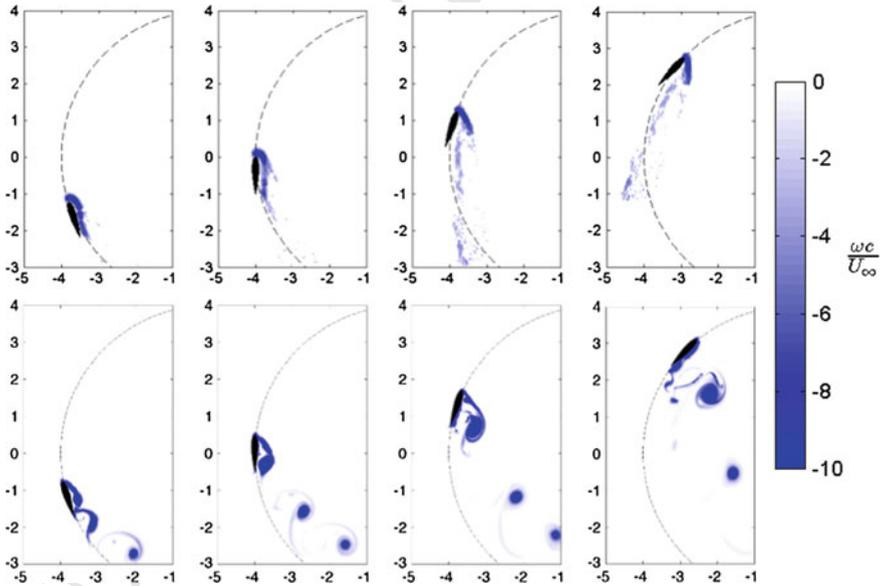
**Fig. 4** Clockwise vorticity contours from experiment  $\text{EPM}^E$  (top) and VAWT computation  $\text{VAWT}^C$  (bottom) at  $\theta = 70^\circ, 90^\circ, 108^\circ$  and  $133^\circ$  respectively from left to right
